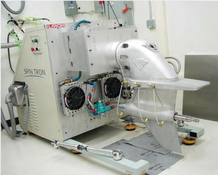
**ABOVE:** Ilmor, the distinguished engine developer for racing cars and boats, test their latest Indy marine outdrive. This new outdrive and accompanying transmission were both developed using the Spintron. "We use our Spintron to validate all our new or improved parts including valve springs, each of which is subjected to a 100-hour test before use." Ian Hawkins, Ilmor Marine.
