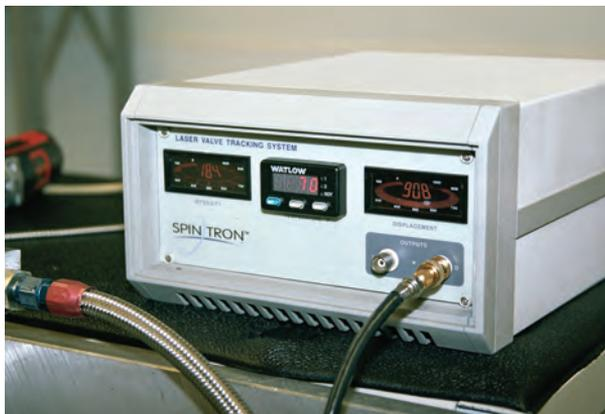
examination until fairly recently. SpinTron changed all of that—the behavior of every component responsible for valve actuation (either OHV or OHC) can now be examined, imaged, and graphed in real time for analysis.
