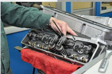
Race engine builders make use of test machines at SpinTron's Michigan facility. The engine on the SpinTron uses a mandrel instead of its original crankshaft and valve train tests are usually conducted on one cylinder.
