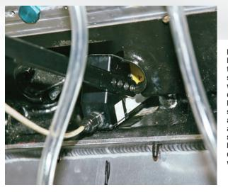
LEFT: Mounted on a tripod to keep it secure and vibration-free during testing, the laser position sensor is placed in a cylinder through an opening in the side of the engine block. Its red laser dot is aimed at a valve head.
