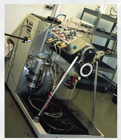
teams use them to gain vital data. Whether they are gathering information on valve train performance or calculating frictional losses within the engine, transmission, or final drive, they are aware that knowledge is power, and having access to SpinTron data is a good first step. "How else can you explore beyond normal mechanical limits of race engine development without provoking a trail of devastation," says SpinTron creator Bob Fox.
