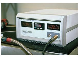
examination until fairly recently. SpinTron changed all of that—the behavior of every component responsible for valve actuation (either OHV or OHC) can now be examined, imaged, and graphed in real time for analysis.
