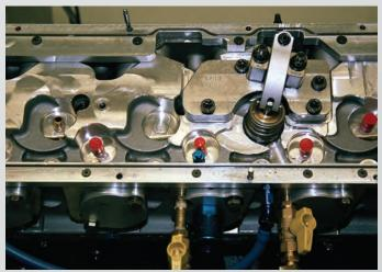
ABOVE: This particular Jesel test requires just one rocker arm and attendant valve train, operating on a single cylinder. Note the blue hose provides cooling oil to the valve spring. The other fittings function as oil drains.
