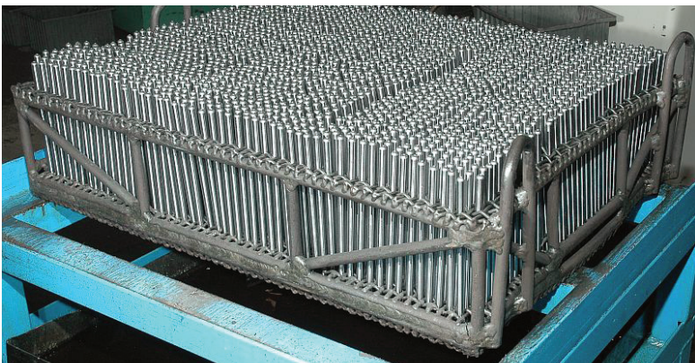
Trend pushrods are stacked in specially constructed stainless-steel racks within 2 degrees of vertical to ensure they remain straight during the heat-treating process, where temperatures reach 1,700 degrees.
