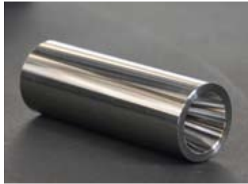
A tapered piston pin is one where the inside diameter is tapered to place the majority of the metal where it will do the most good, in the middle of the pin. This allows for a relatively lightweight pin, which can withstand the pressure.
