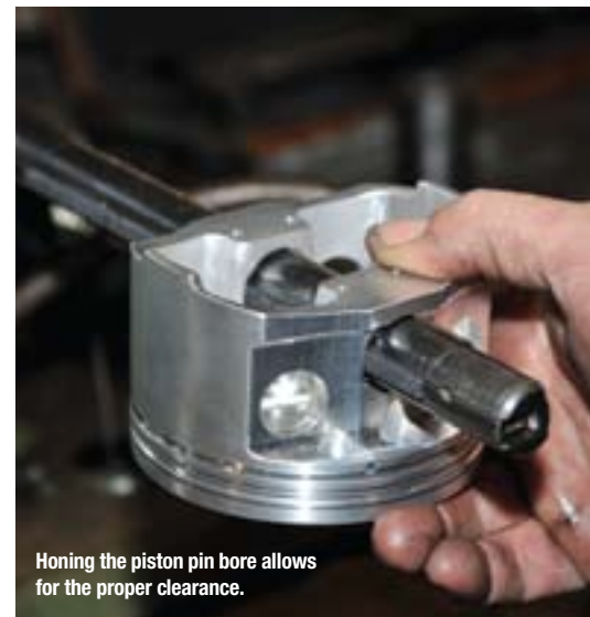
Inserting a piston pin into a piston might seem like an easy task, but the tolerances must be held tight in order to eliminate the piston wobbling on the pin, yet not so tight as to cause galling and seizure.
