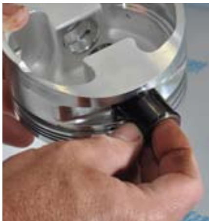
Inserting a piston pin into a piston might seem like an easy task, but the tolerances must be held tight in order to eliminate the piston wobbling on the pin, yet not so tight as to cause galling and seizure.
