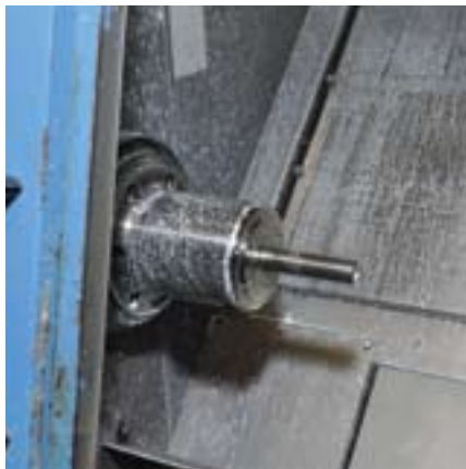
Today, piston pins are manufactured using sophisticated CNC equipment, which can hold tolerances to extremely small numbers. After manufacture, the pin surface is lapped to a mirror finish to alleviate stress risers. In some cases, a coating is also applied to the surface.
