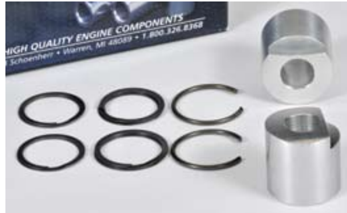
A full-floating piston pin can be held in the piston by a number of methods. From left to right is a single spiral lock, a thicker spiral lock, a wire clip and, finally, buttons made from aluminum that simply ride against the cylinder wall and don't allow the pin to walk out of the piston.
