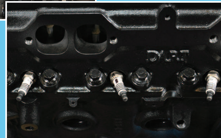
Bottom: The three principal operations that occur in the dyno room are running the break-in procedure with outer valve springs only; checking for cylinder and combustion chamber leaks (known as leak-down testing); and performing the dynamometer test. The leak-down test (pictured) is conducted by applying steady, fixed air pressure to the cylinders. Stoa expects less than five percent leakage. Recently he successfully tested Trend’s new tool-steel solid flat tappets using both inner and outer springs during break-in, thus saving several hours of work.
