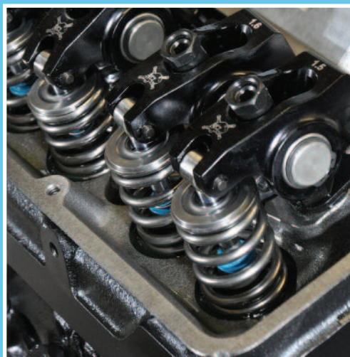
Above: The ratios of stud-mounted rockers are usually altered by moving the pushrod seat or cup further away from the fulcrum (lower ratio) or closer to it (higher ratio). Higher ratios provide greater valve lift and faster valve lift. They also intensify the loading on the pushrod.
