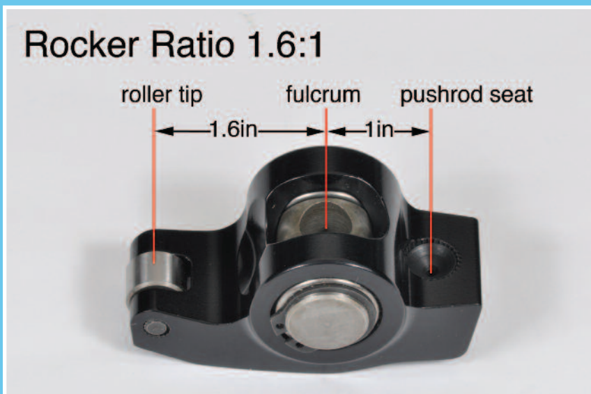
Above: The ratios of stud-mounted rockers are usually altered by moving the pushrod seat or cup further away from the fulcrum (lower ratio) or closer to it (higher ratio). Higher ratios provide greater valve lift and faster valve lift. They also intensify the loading on the pushrod.
