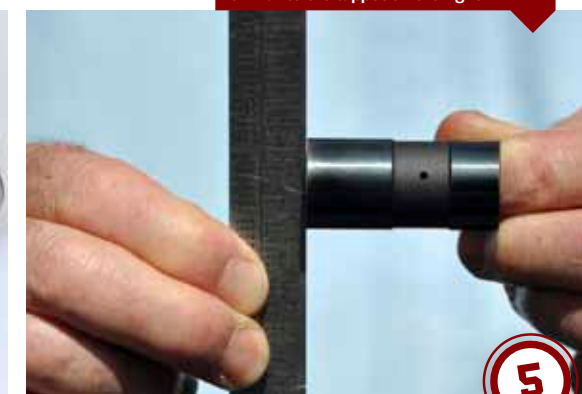
Without the proper rotation of the tappet in its bore, damage can occur similar to the tappet on the right
