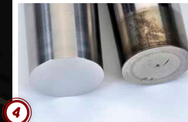
Though barely discernible to the eye, tool steel solid flat tappets, like their cast iron counterparts, have a crown on their contact area approximately 0.0015in high with a radius of 50in to 60in
