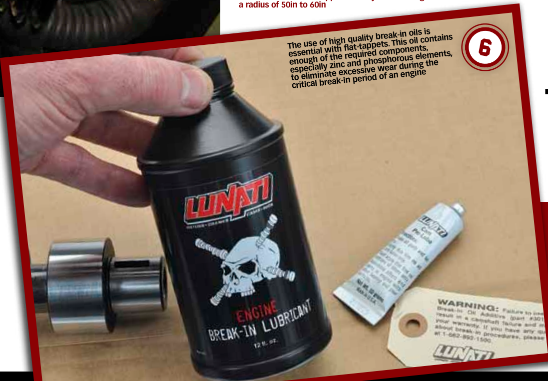
Though barely discernible to the eye, tool steel solid flat tappets, like their cast iron counterparts, have a crown on their contact area approximately 0.0015in high with a radius of 50in to 60in
